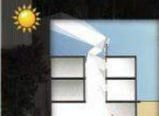
A row white reflector is provided on the roof against the west facade which reflects the light into the class room of the west facade in the morning and it gets illuminated with natural
